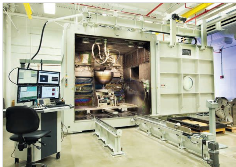
The Sciaky electron beam additive manufacturing machine is the largest 3-D printer in use at Lockheed Martin Space Systems in Denver.
