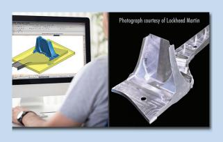
Starting with a 3D model from a CAD program, Sciaky's fully-articulated, moving electron beam gun deposits metal (via wire feedstock), layer by layer, until the part is built and ready for finish machining. Deposition rates typically range from 5 to 25 lbs/hr (2.27 to 11.36 kg/hr), depending upon part geometry and the material selected.
